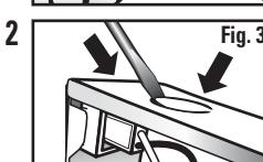
Once you have determined the position the fixture will be mounted, mark the corresponding knock-out closest to the insulated multi-wire end and remove it (Fig. 3). CAREFULLY REMOVE THE KNOCK-OUT BY HAMMERING A FLATHEAD SCREWDRIVER OR PUNCH UNTIL THE SURFACE BREAKS. If the knock-out did not break free, use pliers and bend it back and forth until it snaps off.
