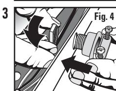
Attach a wire coupling by (not included) inserting the threaded end (from outside the fixture) through the knock-out. Secure the wire coupling to the fixture's chassis by tightening the fastener (from inside the fixture) (Fig. 4). NOTE: Orient the wire coupling in a way that allows the clamp screws to be tightened after the fixture has been attached to the mounting surface.
