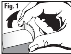
Remove the diffuser by pulling back and up on the top edge of the diffuser using your fingertips (**Fig. 1**).
