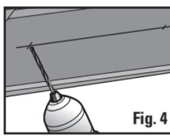
Using a small drill or nail, make two small starter holes at the marked locations (**Fig. 4**).
