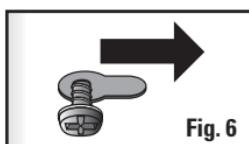
Slide the fixture over until the narrow legs of the keyhole slots are under the heads of the screws (**Fig. 6**). Finish tightening the screws until they are firmly seated, and the fixture is tightly secured to the mounting surface.
