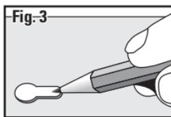
Place fixture up to mounting surface and mark position of the narrow end of the keyslot holes on the mounting surface with a pencil (**Fig. 3**). The screw hole locations must be exact for the fixture to mount properly.
