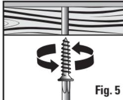
Screw in the two #8 mounting screws until there is approximately 1/8" of space remaining under the head of the screw (**Fig. 5**).
