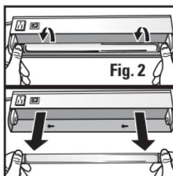
Remove the bulb from the fixture by placing your thumbs on the metal ends of the bulb. While applying slight pressure on the bulb, roll the bulb toward you until the contact pins on the ends of the bulb disengage from the socket. Pull the bulb straight out from the socket and set aside during mounting (**Fig. 2**).
