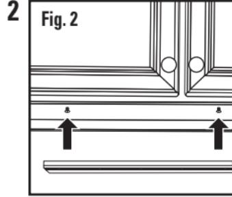
Position the fixture over the wood screw heads. Slide the fixture over so the wood screw heads engage the narrow section of the keyhole slots (Fig. 2). If the fixture still seems loose, remove the fixture and tighten the wood screws another 1/4 turn. Once the fixture is securely mounted, insert the power cord to the fixture and then plug into the wall outlet.
