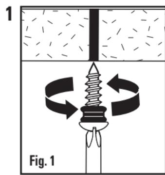
Using a small drill or nail, make two small pilot holes at the marked locations. Place a grommet over each wood screw. Drive in the two wood screws until the grommets contact the bottom of the mounting surface. Then turn the screws another 1/4 turn (Fig. 1). The screws must be driven in straight for the fixture to mount properly.
