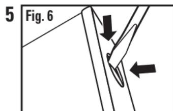
Determine which corresponding knock-out is closest to the supply wire feed and remove it. CAREFULLY REMOVE THE KNOCK-OUT BY HAMMERING IT WITH A FLATHEAD SCREWDRIVER OR PUNCH UNTIL THE SURFACE BREAKS (Fig. 6). If the knock-out does not break free, use pliers and bend it back and forth until it snaps off.
