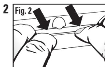
To open the wire compartment cover, disengage both chassis locking tabs by pushing in the side of wire compartment cover (Fig. 2) and lifting it up to expose the wire connections and hardware kit inside (Fig. 3).
