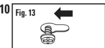
Slide the fixture over until the narrow ends of the keyhole slots are under the heads of the wood screws (**Fig. 13**). Finish tightening the wood screws until they are firmly seated and the fixture is tightly secured to the mounting surface.
