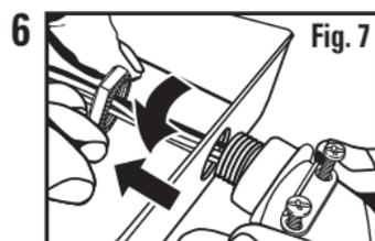
Attach the strain relief by inserting the threaded end through the knock-out (Fig. 7). Secure the strain relief to the fixture by tightening the fastener to the threaded tube. **NOTE:** Remember to have the strain relief screws oriented in a manner that allows tightening/loosening of the clamp after the fixture has been attached to the mounting surface.
