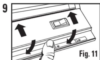
Re-attach the wire compartment cover by hinging the cover with the fixture chassis and closing (**Fig. 11**). Press on the cover and secure the front lip under the locking tab (**Fig. 12**).
