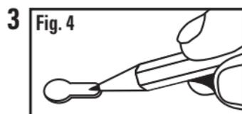
Mark the general area to install the fixture. Locate the mounting keyhole slots on the back of the fixture. Mark the corresponding placement on the mounting surface (Fig. 4).
