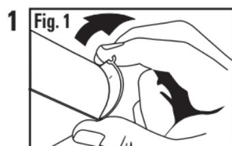
Remove the diffuser by pulling back and up on the top edge (Fig. 1).
