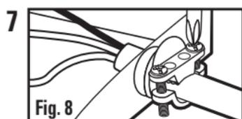
Insert a flexible whip or NM cable (not included) through the strain relief and tighten the clamp until it is secure (**Fig. 8**). Allow enough wire length to make the connection. **WARNING:** Make sure the POWER is OFF.
