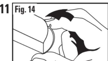
Re-install the diffuser (**Fig. 14**).
