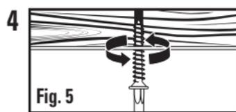
Use an awl or nail to dimple the screw holes or drill a 1/16 in. pilot hole into the marked locations. Tighten the screws leaving 1/2 in. of the screw protruding from the surface (Fig. 5).
