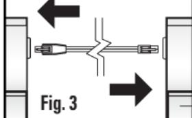
Link additional fixtures by following the linking instructions outlined in steps 1 and 2 (**Fig. 3**). Once all fixtures have been linked, insert the power cord connector plug into the power port on the end of the last fixture and the grounded plug into the outlet. **NOTE:** Each light can be individually operated by the on/off switch located on each fixture.
