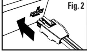
**NOTE:** The linking cord is fitted with a distinct cord connector plug at each end and will only connect one way. Try inserting one end of the linking cord into the power port, if that fails try the other end of the linking cord (**Fig. 2**). DO NOT try to force the plug into the port. When correctly inserted the catch on the top of the cord connector plug will click into the power port.
