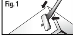
Using a flathead screwdriver, carefully pry off the plastic cap that covers the power port on the fixture (**Fig. 1**).
