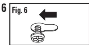
Slide the fixture over until the narrow ends of the keyhole slots are under the heads of the wood screws (Fig. 6). Finish tightening the wood screws until they are firmly seated and the fixture is tightly secured to the mounting surface.
