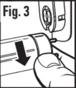
Remove the bulb from the fixture by placing both thumbs on the metal ends of the bulb (Fig. 2). While applying slight pressure on the metal ends, roll the bulb forward until the contact pins on the ends of the bulb disengage from the socket (Fig. 3). Pull the bulb straight out from the socket and set aside.
