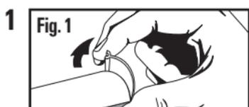
Remove the diffuser by pulling back and up on the top edge of the diffuser (Fig. 1).
