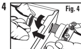
4 Attach the strain relief by inserting the threaded end through the knock-out (Fig. 4). Secure the strain relief to the fixture by tightening the fastener to the threaded tube. **NOTE:** Remember to have the strain relief screws oriented in a manner that allows tightening/loosening of the clamp after the fixture has been attached to the mounting surface.
