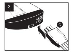
4. Insert the opposite end of the linking cord into the "Power-In" port of the additional unit. **NOTE:** Each light can be individually operated by the on/off switch located on each fixture.
