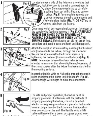
bundled with the supply wires. Insert the end of that ground wire into the open hole in the push-in connector (**Fig. 11**). If unsure whether or not the electrical system is properly grounded, or the flexible whip or NM cable is connected to an electrical box that is plastic and has no ground wire, or are unfamiliar with the methods of properly grounding the fixture, consult a qualified electrician.
