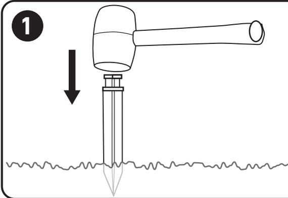
To mount the light with the included stake, use a mallet to insert stake into the ground. **DO NOT USE HAMMER.**
