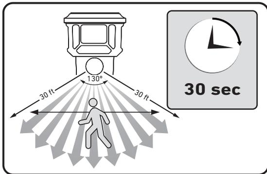
The light is activated when the motion sensor detects movement. The sensor detects motion in a 130° coverage zone for up to 30 feet. The sensor is most effective from side-to-side motion, rather than motion coming straight at it (in-and-out). The "time on" for the light is 30 seconds after each time motion is detected during night hours.
