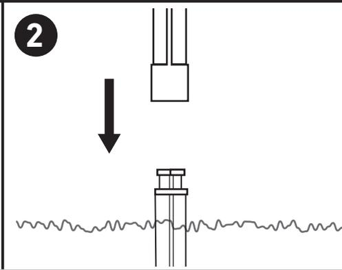
Insert post onto the ground stake.
