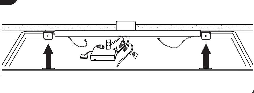
**5A** Keeping the support wire hooks attached to the mounting plate, lift up the LED panel, being careful not to scratch ceiling. Align and insert the 2 metal tabs (on the same side of the mounting plate as the support wires) into the corresponding slots on the LED panel.
