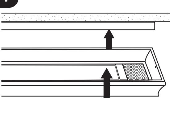
**5C** Slide panel until tabs are locked into place. Note that the direction will be either left or right, depending on panel orientation.
