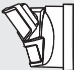
**THE FIXTURE USES A PASSIVE INFRARED (PIR) MOTION SENSOR AND AS SUCH DETECTS CHANGES IN INFRARED RADIATION OF WARM OBJECTS MOVING ACROSS THE DETECTION ZONES.**
