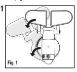
Remove the security light from the rear housing cover by gripping the fixture and turning counter clockwise until the catches disengage from the rear housing cover (**Fig. 1**).
