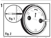
Remove the mounting base by turning counter clockwise until it comes loose. For mounting to concrete or masonry, install the anchors, by drilling two 3/16-in. pilot holes into the mounting surface. Insert the anchors into the holes and tap them into place so they are flush with the surface (Fig. 1). Place the rear housing cover, with the writing facing away from the wall, over the mounting location and secure the rear
