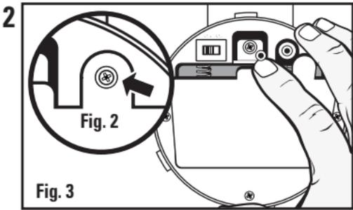
Remove the screw on the battery compartment cover (Fig. 2). With fingertips, pull up on the battery compartment catch and pull outward to remove the battery compartment cover (Fig. 3).
