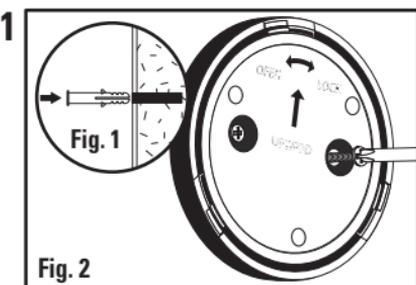
Remove the mounting base by turning counter clockwise until it comes loose. For mounting to concrete or masonry, install the anchors, by drilling two 3/16-in. pilot holes into the mounting surface. Insert the anchors into the holes and tap them into place so they are flush with the surface (Fig. 1). Place the rear housing cover, with the writing facing away from the wall, over the mounting location and secure the rear housing cover to the mounting surface with wood screws (Fig. 2).
