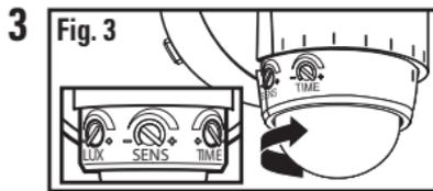
3 The control knobs for adjusting the operation of the security light (TIME, SENS and LUX) are located on the back side of the motion sensor. To gain access to these controls, rotate the sensor clock-wise (Fig. 3).
