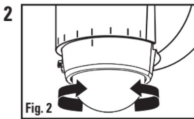
2 The motion sensor can be rotated to position in the direction of an area to be covered. If the 2 tick marks are aligned, the motion sensor is focused straight ahead. The motion sensor can be rotated approximately 45 degrees right or left of center (Fig. 2). The motion sensor has a maximum detection field of 130° at a distance of 30 ft.
