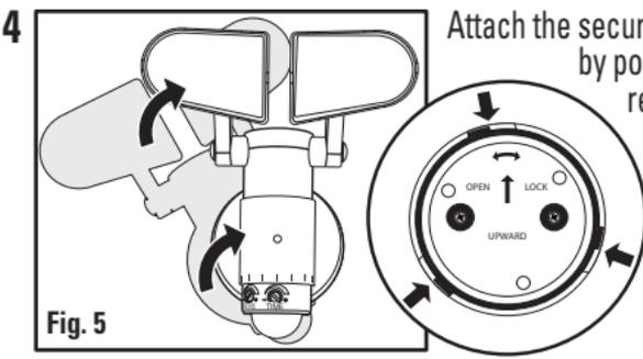
Attach the security light to the rear housing cover by positioning the security light over the rear housing cover at an angle. Engage the security light into the grooves of the rear housing cover and secure by twisting clockwise until the security light is seated vertically (Fig. 5).
