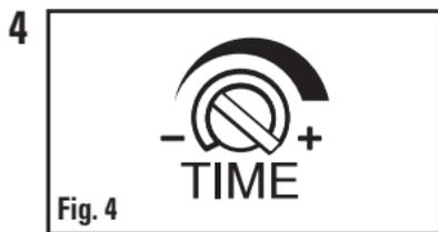
4 The TIME control knob can be adjusted to control the length of time the light stays ON when triggered by the PIR sensor (Fig. 4). In the far left position (-), the duration time is approximately 10 seconds. In the far right position (+) the duration time is approximately 30 seconds.
