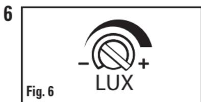
6 The LUX control knob can be adjusted for the surrounding level of darkness needed to activate the PIR (Fig. 6). This is quite variable. The far left position (-) sets for maximum level of darkness (or near full darkness). The far right position (+) sets for minimum level of darkness.
