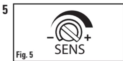
5 The SENS control knob can be adjusted to control the range of the PIR sensor (Fig. 5). The far left position (-) sets the PIR sensor range to approximately 1 foot. The far right (+) sets the PIR range to approximately 30 feet.
