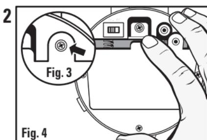
Remove the screw on the battery compartment cover (Fig. 3). With your fingertip, pull up on the battery compartment catch and pull outward to remove the battery compartment cover (Fig. 4).
