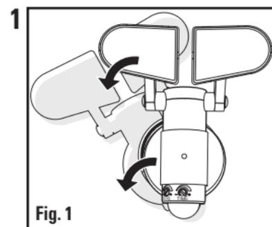
1 Remove the security light from the rear housing cover by gripping the fixture and turning counter clockwise until the catches disengage from the rear housing cover (Fig. 1).
