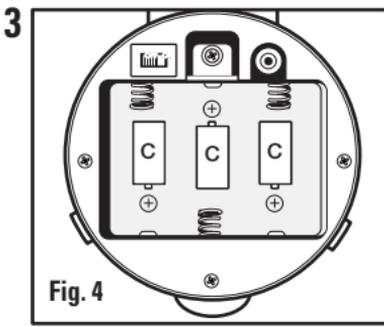
Insert 3 new alkaline C cell batteries (not included) into the battery compartment according to the "+" and "-" markings near the battery drawings (Fig. 4). Re-attach the battery compartment cover by aligning the legs on the lower edge of the battery compartment cover onto the fixture body and close the cover until the catch at the top engages. Replace the screw. Do not mix old and new batteries. Cold weather may have a negative impact on battery life.
