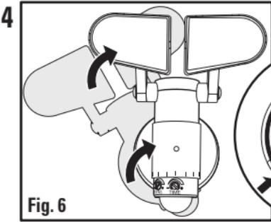
4 Attach the security light to the rear housing cover by positioning the security light over the rear housing cover at an angle. Engage the security light into the grooves of the rear housing cover and secure by twisting clockwise until the security light is seated vertically (Fig. 6).
