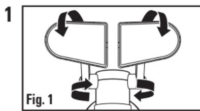
1 The individual light heads can be adjusted side to side and up/down independently to aim the light heads in the direction desired (Fig. 1).
