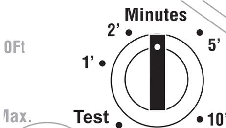
The **MINUTES** control determines the length of time the lights stay on. When the **MINUTES** control is set between 1 and 10, the light will only come on during night time hours.
