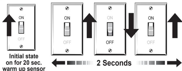
**MANUAL OVERRIDE** allows the light to turn on at any time, by overriding all sensor controls, so the light comes on regardless of time of day.
