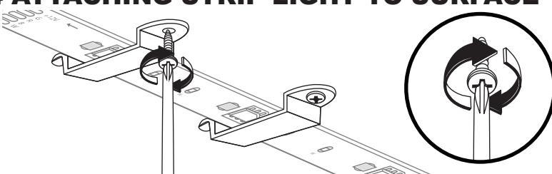
Hold Strip light to desired location. Place mounting clips carefully over the Strip light and screw in to the surface careful not to screw into the Strip light.
