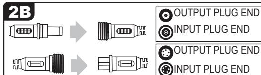
The two different cords have two different ends: one input and one output. Insert the **OUTPUT PLUG END** into the **OUTPUT CONNECTOR** of the preceding fixture and insert the **INPUT PLUG END** into the **INPUT CONNECTOR** of the fixture being added. Twist the water tight connection piece until completely tightened.
