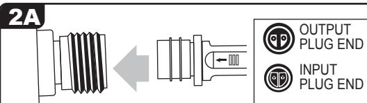
The plug and cord have two different ends: one input and one output. Line up the arrow, and Insert the **OUTPUT PLUG END** into the **OUTPUT CONNECTOR** of the preceding fixture and insert the **INPUT PLUG END** into the **INPUT CONNECTOR** of the fixture being added. Twist the water tight connection piece until completely tightened.
