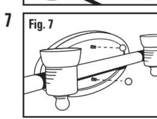
Pull any excess wire up from the fixture and through the center hole of the mounting bracket. Push the excess supply wires back into the electrical box or under the canopy. Move the mounting plate up to and over the mounting screws and screw on both base fasteners on opposite sides of the mounting base (Fig. 7). Hand-tighten the round fixture fasteners until the pan is securely against the wall. Make sure not to pinch any of the wires under the pan.
