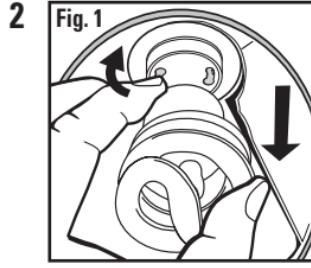
Remove the old bulb by grasping it firmly at the plastic base of the bulb and firmly twist the bulb counter-clockwise until it "unseats" and lines up with the large end of the openings (**Fig. 1**). Pull straight up. Be careful not to drop the bulb.
