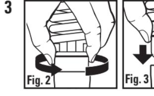
Grasp the replacement bulb in the same manner and re-insert the replacement bulb into the socket and twist the bulb clockwise until it "seats" (**Fig. 2 and Fig. 3**). Do not force the bulb into the socket or twist forcefully.
