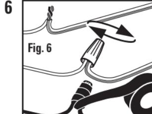
Tighten the wire nuts properly to prevent the wires from coming loose (Fig. 6). Tape the wire nuts to the wire using electrical tape. Carefully push the excess wires back inside the electrical box.
