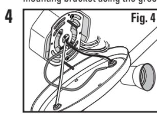
Pull both sets of the fixtures' wires through the center hole of the mounting bracket (Fig. 4). Cut off the excess wire that you have pulled through, leaving six (6) inches (15,2 cm) for electrical connections and make sure that 1/2 in. (1,3 cm) of the insulation has been stripped off. Pull any excess wire up from the fixture and through the center hole of the mounting bracket. Push the excess supply wires back into the electrical box or under the mounting base.
