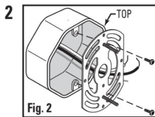
Using the old electrical box screws, secure the mounting bracket to the electrical box, make sure the protruding machine screws are parallel to the floor (Fig. 2). Pull the existing supply wires around the sides of the mounting bracket. Do **NOT** pull the supply wires through the center hole of the mounting bracket. You may need to use the slots to mount the universal bracket so the long machine screws are parallel to the floor. This will allow for leveling of the fixture.
