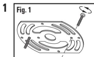
Screw the long machine screws (included) into the threaded holes on the mounting bracket (Fig. 1). If your mounting bracket has more than 2 threaded holes, measure the center-to-center distance of the holes to make sure it matches the hole openings in the pan of your fixture.
