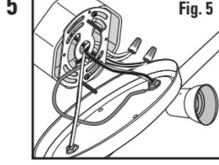
Connect the supply leads from the electrical box to the fixture wire leads using the medium wire nuts supplied in your installation hardware kit as per the illustration (Fig. 5). The black lead from the fixture goes to the black supply lead and the white lead from the fixture goes to the white supply lead.
