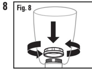
While holding the glass diffuser, secure the diffuser by screwing on the diffuser locking ring in a clockwise direction (Fig. 8). Hand-tighten the diffuser locking ring until it is on tightly and the diffuser is held securely in place. **CAUTION: DO NOT OVER-TIGHTEN!** Over-tightening may cause the diffuser to crack.
