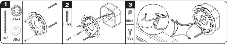
Screw the two long machine screws (II) through the threaded holes from the backside of the mounting bracket (AA). On the front side of the mounting bracket (AA), secure the hex nuts (DD) onto the screws until they are flush with the mounting bracket (AA).
