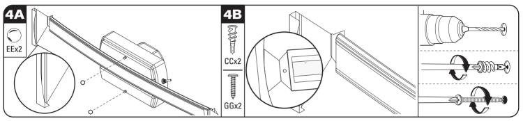
Before mounting fixture, make sure the closed catches of the diffuser channel are on the bottom to prevent the diffuser from falling out. Secure the fixture to the electrical box with the screw caps (EE). The back plate should be tight against the wall surface.
