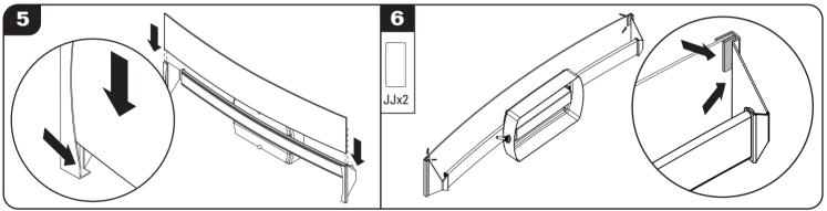
5 Simultaneously, slide both ends of the diffuser evenly into the channels at each end. **NOTE**: The plastic diffuser, when properly installed, is meant to have an arc spaced away from but aligned with the LED board. If the diffuser does not line up with the LED board, carefully bend the ends in or out slightly in order to align. Once both ends of the diffuser are set in the openings of the end caps, carefully push/pull the diffuser into place until it is securely seated in the closed catches.
