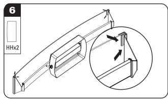
In order to hold the diffuser in place, insert the silicone pads (HH) between the diffuser and the end cap channel at each end. Restore power to the fixture.
