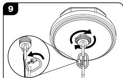
Re-attach quick link to the collar mounting stem of the fixture. Raise canopy until collar mounting stem passes through its center and secure by tightening the collar lock ring. Restore power to the fixture.
