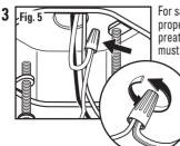
For safety and proper operation, the fixture must be properly grounded. A green or bare copper ground wire is preattached to the fixture pan. The fixture ground wire must be spliced to the green or bare copper ground wire in the electrical box using one of the wire nuts
