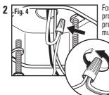
For safety and proper operation, the fixture must be properly grounded. A green or bare copper ground wire is preattached to the fixture pan. The fixture ground wire must be spliced to the green or bare copper ground wire in the electrical box using one of the wire nuts
