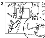
Connect the supply leads from the electrical box to the fixture wire leads using the wire nuts (Fig. 5). The connections need to be made on the back side of the pan. The black lead from the fixture pan is spliced to the black supply lead, and the white lead from the fixture
