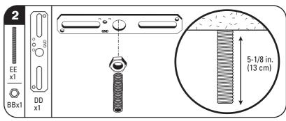
Attach the threaded tube (EE) to threaded hole in the center of the mounting bracket (DD). Lock the tube in place using the hex nut (BB). The threaded tube should extend below the ceiling line. 5-1/8in.(13 cm)
