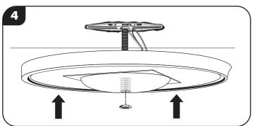
Lift the fixture up to ceiling, carefully guiding the threaded tube mounted on the electrical box into the center hole of the fixture pan.
