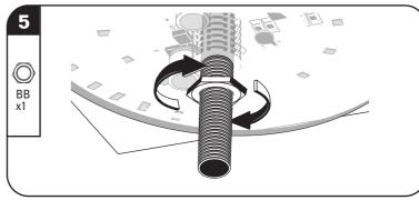
Secure the fixture to the electrical box by tightening down the hex nut (BB) on the threaded tube. DO NOT overtighten. Doing so could fracture the LED lens.
