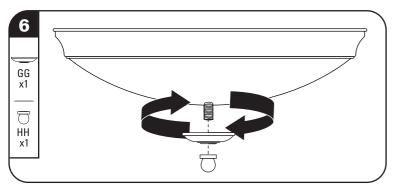
Place the diffuser over the threaded tube, and while holding the diffuser in place with one hand, place the diffuser cap (GG) over the threaded stem, and secure both the diffuser cap, and diffuser with the finial (HH). Restore power to the electrical box to make sure the fixture is working properly.
