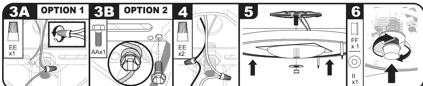
**3A** Option 1: The fixture must be properly grounded. If the J-box has a ground wire, connect the fixture ground wire to the ground wire in the J-box using wire nut (EE). Ground wires are normally green or bare copper.
