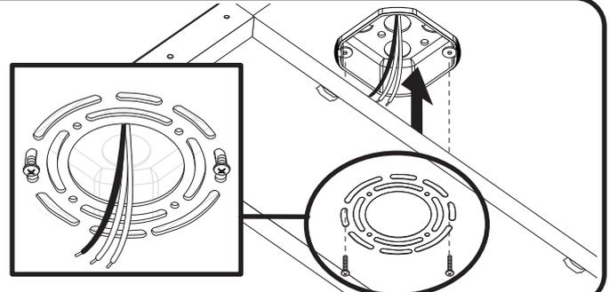
**1** Remove mounting plate from LED panel by sliding into the direction of the slots closest to the mounting screws (AA), and then lifting up. Hold the mounting plate up to the junction box in the desired fixture mounting orientation. Pull black, white and ground supply wires from electrical box through the hole in center of mounting plate. Ground wires can be either green or bare copper. Attach mounting plate to the electrical box using mounting screws (AA) provided.
