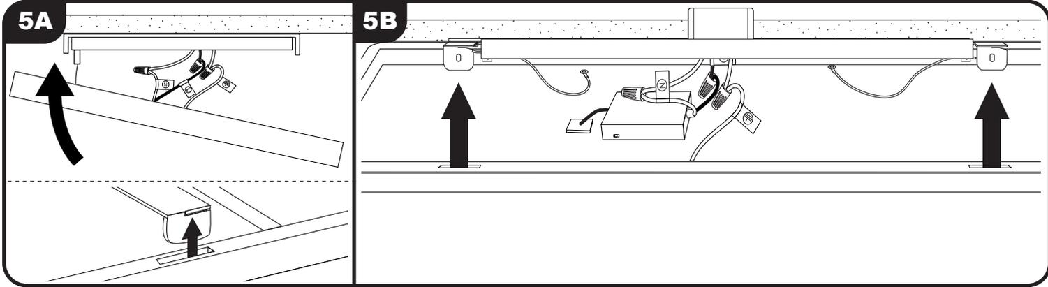
**5A** Keeping the support wire hooks attached to the mounting plate, lift up the LED panel, being careful not to scratch ceiling. Align and insert the 2 metal tabs (on the same side of the mounting plate as the support wires) into the corresponding slots on the LED panel.
