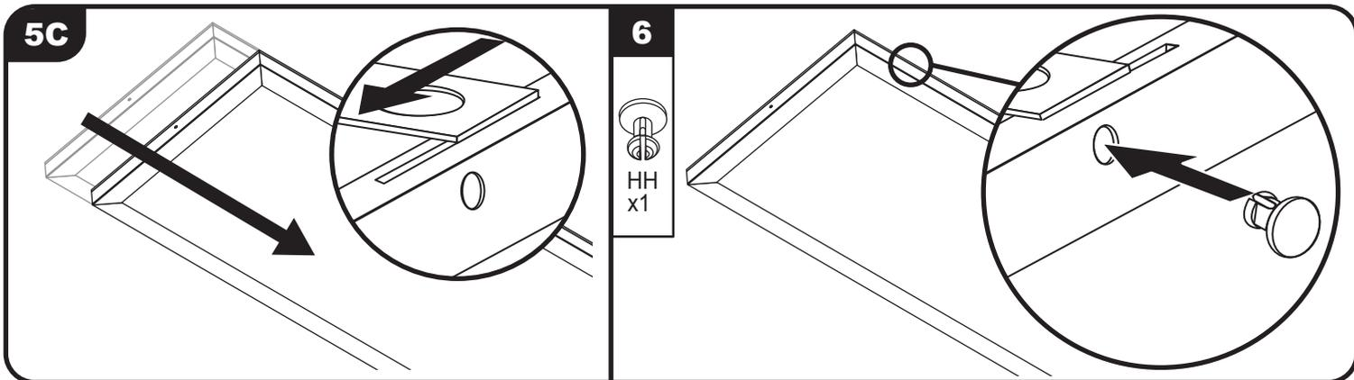
**5C** Slide panel until tabs are locked into place. Note that the direction will be either left or right, depending on panel orientation. Slowly release fixture, making sure it stays in place.
