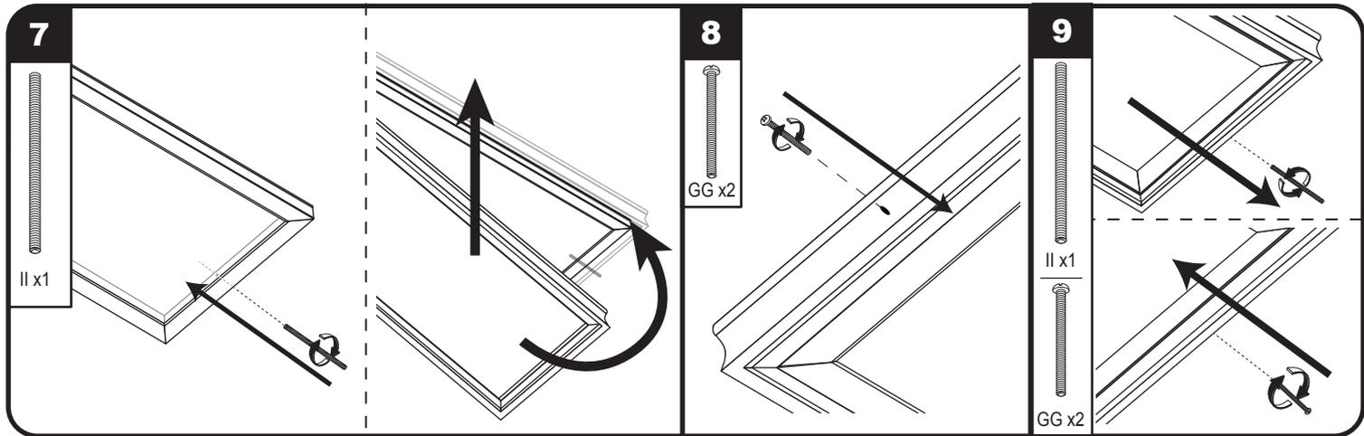
**7** To assist with attaching the frame to flat panel, screw the assist screw (II) into one of the two pre-drilled holes on flat panel. Bring wood frame up to ceiling and place over flat panel and through the assist screw (II). **NOTE:** Make sure the two pre-drilled holes at each end of the frame are closest to the ceiling. The frame should fit closely around the flat panel.
