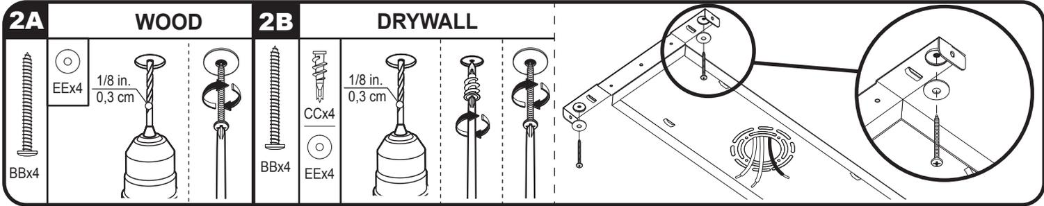
**2A** Locate the open holes for mounting at the corners of the mounting plate and drill 1/8 in. pilot hole in the center. If a wooden stud is encountered, use the wood screws (**BB**) and washers (**EE**) provided to secure the mounting plate directly to stud.
