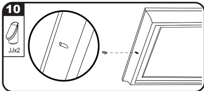
**10** Restore power to the electrical box and verify the light is functioning properly. If the light functions properly, fasten the silicone cap (JJ) into the mounting screw opening.
