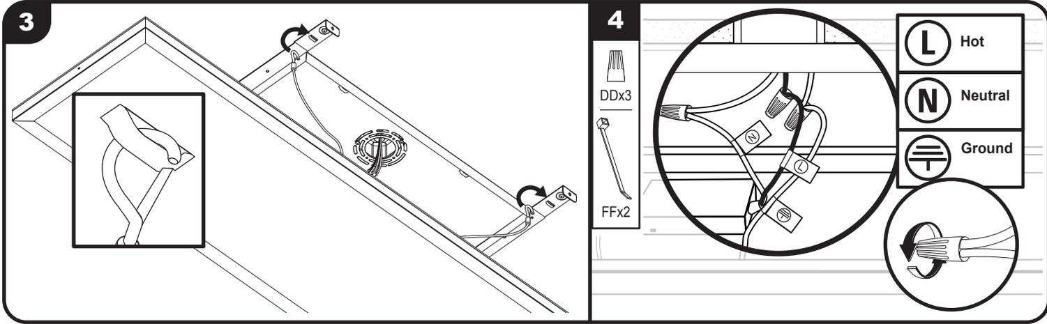
**3** Hold fixture up to secured mounting plate and attach the support wire hooks from the backside of fixture to specially designed slots in mounting plate to temporarily hold fixture for wiring.
