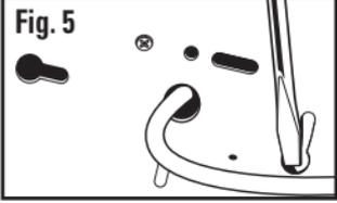
If the keyhole slots are not punched through, remove the appropriate knockouts from the back side of the fixture pan that correspond to the positions of the mounting screw heads on the mounting bracket (Fig. 5). This can be done using a flathead screwdriver and pliers.
