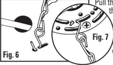
Pull the fixture wires through the hole in the center of the fixture pan to the backside of the fixture. Using the support chain, connect one end to the back of the fixture pan near the center in the specially designed slots (Fig. 6) Hook the other end of the support chain to the electrical box (Fig. 7). This will allow for a hands free support for wiring.
