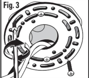
Remove the existing screws from the electrical box. Pull the supply wires from the electrical box through the center hole of the mounting bracket. Attach the mounting bracket to the electrical box, using the electrical box screws removed earlier. Both long machine screws installed in Step 1 should be oriented with both screwheads facing toward the floor and they be aligned with the center run of the fixture position (Fig. 3).
