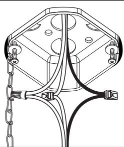
**2** Fixture must be properly grounded. Connect fixture ground wire to ground wire in electrical box using wire nut (**BB**). These wires can be either green or bare copper. Insert black supply lead into connector on black fixture wires and white supply lead into connector on white fixture wires. Push excess wire into electrical box.
