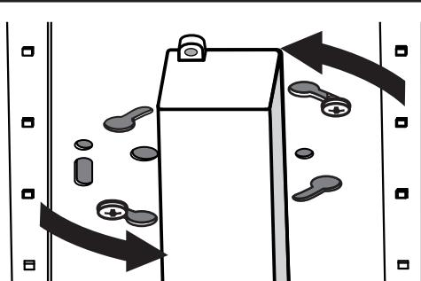
**3** Remove support chain. Insert both screwheads into keyhole slots and rotate fixture pan. Once screws are engaged, maneuver fixture into desired position. Tighten screws.
