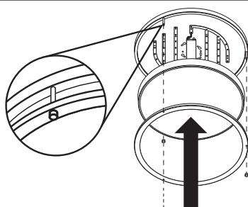
**4** Place diffuser and decorative ring against fixture pan. Once holes are aligned, hold both diffuser and ring in place and attach post caps to secure decorative ring. Restore power.
