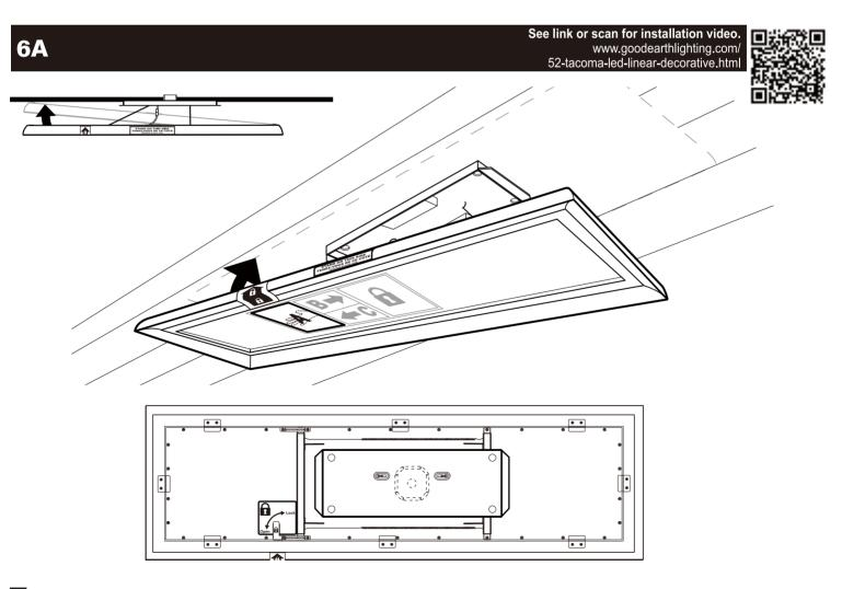
6A Place hand over handprint in Box A and lift this side up to the ceiling, being careful not to scratch ceiling.
