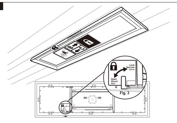
Slowly release fixture making sure it stays in place. To lock the fixture in place, extend hand over the frame above the lock arrow and rotate the rail locking lever into place (**Fig. 3**). If lever does not rotate fully into place, the panel is not positioned properly. Manuever fixture until it seats properly or repeat mounting steps if needed until locking lever rotates into place.
