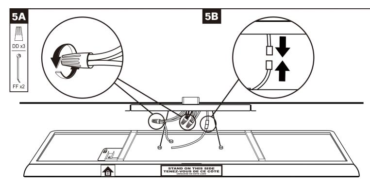
Fixture must be properly grounded. Connect mounting plate ground wire and fixture ground wire to green or bare copper ground wire in electrical box using wire nut (**DD**).
