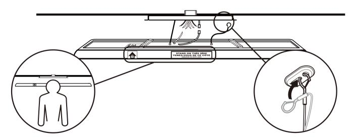
4 Stand on the side of fixture where the lock indicated with an arrow on the frame is located. Getting help if needed, hold fixture up to secured mounting plate and attach the support wire hooks from the backside of fixture to specially designed slots in mounting plate. **NOTE:** Insert hook into large slot and out the smaller hole. Allow fixture to hang, tilted to one side, for wiring.
