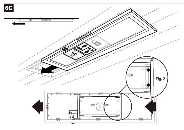
With the fixture fully engaged with the mounting plate, slide the fixture back to the opposite side (Box C), allowing the fixed rail to hook the other end of the mounting plate (Fig. 2).
