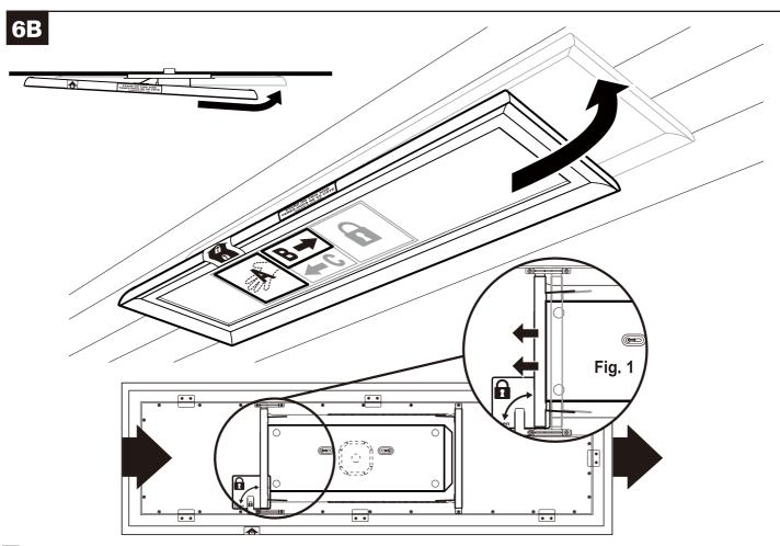
Keeping one hand on **Box A**, slide fixture over (**Box B**) while raising the other end of the fixture up to the ceiling. You should feel the rail on the fixture hook the edge of the mounting plate and slide to the open position (**Fig. 1**).
