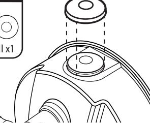
**5** The fixture comes with a built in Dusk-to-Dawn sensor. If the security light cycles ON and OFF, the Dusk-to-Dawn sensor may be activating due to reflected light from a nearby surface. Place the directional sensor cap (HH) firmly over the Dusk-to-Dawn sensor. This should prevent extraneous light from "tripping" the Dusk-to-Dawn sensor.
