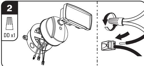
**2** Fixture must be properly grounded. Connect fixture ground wire to ground wire in electrical box using wire nut (DD). These wires can either be green or bare copper. Insert black supply lead into connector on black fixture wires and white supply lead into connector on white fixture wires. Push excess wire and wire connections back into electrical box. Orient light head properly to prevent water from damaging the fixture.
