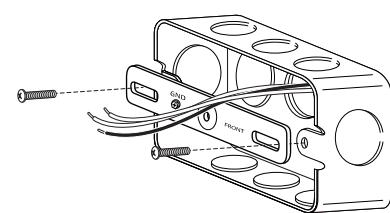
**1S** Pull supply wires out of the junction box (j-box). With the side marked "FRONT" facing out, attach the mounting strap (FF) to the j-box with machine screws (AA or BB). Remove the protective liner from adhesive side of the gasket (GG). Guide the j-box wires through the gasket opening. Align the center holes of the gasket and mounting strap and apply the gasket to the outer edge of round j-box.
