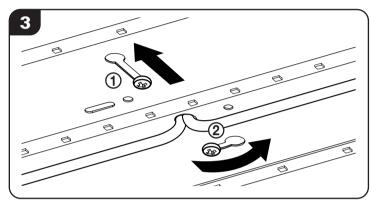
3 Remove support chain. Insert first screwhead into straight keyhole slot ①, pivot fixture and insert second screw into curved keyhole slot ②. Once screws are engaged, maneuver fixture into desired position. Tighten screws.
