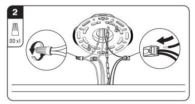
2 Fixture must be properly grounded. Connect fixture ground wire to ground wire in electrical box using wire nut (DD). The ground wires can be either green or bare copper. Insert black supply lead into connector on black fixture wires and white supply lead into connector on white fixture wires. Push excess wire into electrical box.
