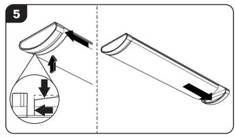
Depress middle of diffuser as you slide one end into an endcap.
