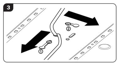
Remove support chain. Insert first screwhead into straight keyhole slot (1), pivot fixture and insert second screw into curved keyhole slot (2). Once screws are engaged, maneuver fixture into desired position. Tighten screws.
