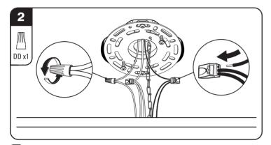
Fixture must be properly grounded. Connect fixture ground wire to ground wire in electrical box using wire nut (DD). The ground wires can be either green or bare copper. Insert black supply lead into connector on black fixture wires and white supply lead into connector on white fixture wires. Push excess wire into electrical box.
