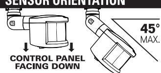
The (PIR) sensor head must be oriented specifically to prevent water from entering.
