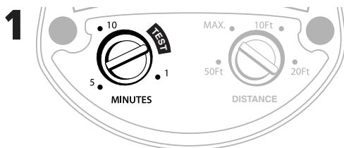
When the **MINUTES** control is set to **TEST**, the light will operate both during daylight and night time.
