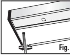
**Fig. 4** Once fixture is secured to cabinet replace the wire compartment cover (**Fig. 4**). Plug in the power cord and the installation is complete.
