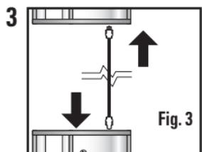
If a second or third fixture are being installed simply connect to a previously installed fixture, follow the instructions outlined in Steps 1 and 2. Make sure the power is off before connecting additional fixtures. Also, make sure that the distance between fixtures does not exceed the connector cord length (Fig. 3).
